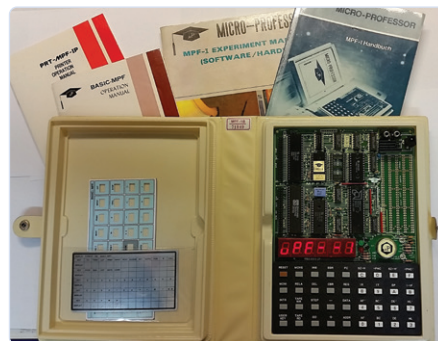
Figure 1: The Micro-Professor MPF-1B in the opened book housing and the related documentation.
