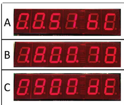
Figure 5: A: Input value 81_{dec} in register BC. B: Start address. C: Result 9 in register DE.
