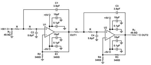
Figure 55. 4-Pole Sallen-Key Low-Pass Filter (ADA4817-2)
