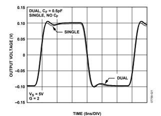
Figure 23. Small Signal Transient Response
