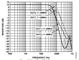
Figure 54. Low-Pass Filter Response
