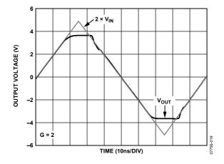
Figure 22. Output Overdrive Recovery
