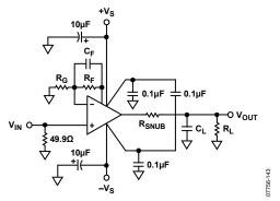
Figure 45. R<sub>SNUB</sub> or C<sub>F</sub> Used to Reduce Peaking
