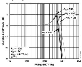
Figure 47. Small Signal Frequency Response for Various Rs (SOIC)
