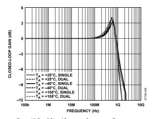
Figure 17. Small Signal Frequency Response vs. Temperature
