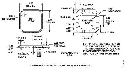
Figure 60.16-Lead Lead Frame Chip Scale Package [LFCSP\_VQ] 4 mm × 4 mm Body, Very Thin Quad (CP-16-4) Dimensions shown in millimeters
