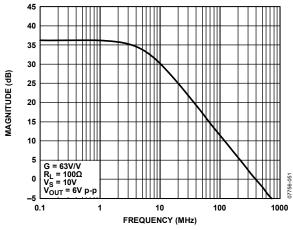
Figure 52. Photodiode Preamp Frequency Response
