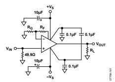
Figure 38. Noninverting Gain Configuration
