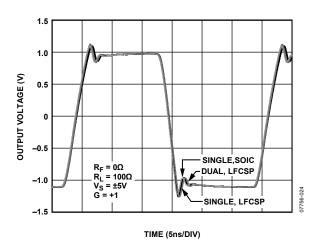
Figure 24. Large Signal Transient Response
