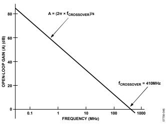
Figure 43. Open-Loop Gain vs. Frequency and Basic Connections
