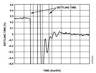
Figure 25. 0.1% Short-Term Settling Time
