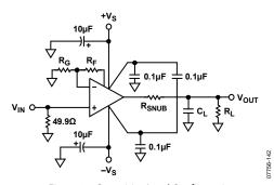
Figure 37. Capacitive Load Configuration
