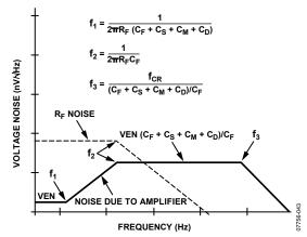
Figure 51. Photodiode Voltage Noise Contributions
