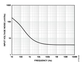
Figure 30. Input Voltage Noise
