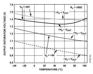
Figure 32. Output Saturation Voltage vs. Temperature
