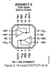
With a wide supply voltage range from 5 V to 10 V and the ability to operate on either single or dual supplies, the ADA4817-1/ ADA4817-2 are designed to work in a variety of applications including active filtering and ADC driving.
