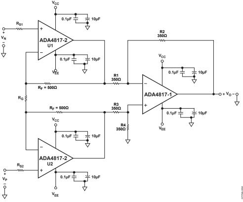
Figure 53. High Speed Instrumentation Amplifier
