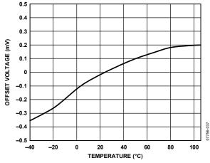
Figure 29. Offset Voltage vs. Temperature
