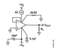
Figure 36. Positive Power Supply Rejection
