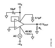
Figure 39. Negative Power Supply Rejection
