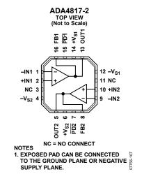
Figure 7. ADA4817-2 Pin Configuration (16-Lead LFCSP)
