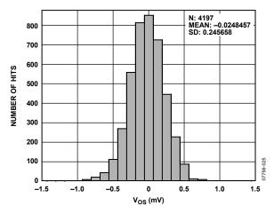
Figure 34. Input Offset Voltage Histogram
