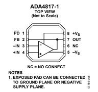
Figure 5. ADA4817-1 Pin Configuration (8-Lead LFCSP)
