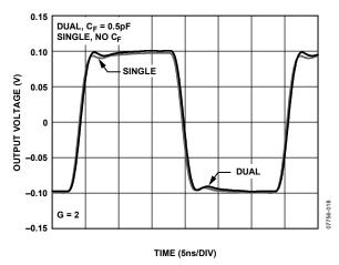
Figure 20. Small Signal Transient Response
