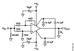
Figure 40. Common-Mode Rejection
