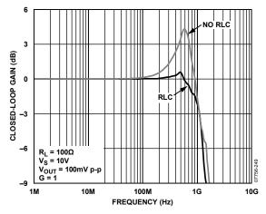
Figure 49. Frequency Response with RLC Circuit
