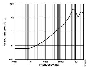
Figure 28. Output Impedance vs. Frequency
