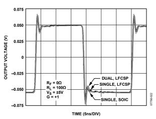
Figure 21. Small Signal Transient Response vs. Package
