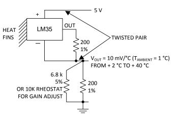
Figure 17. Two-Wire Remote Temperature Sensor (Output Referred to Ground)
