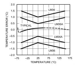
Figure 15. Accuracy vs Temperature (Ensured)
