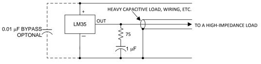
Figure 13. LM35 with R-C Damper
