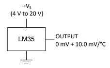
Figure 14. Basic Centigrade Temperature Sensor (2 °C to 150 °C)
