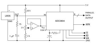
Figure 25. Temperature to Digital Converter (Parallel TRI-STATE Outputs for Standard Data Bus to μP Interface) (128°C Full Scale)
