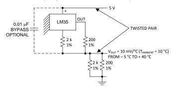
Figure 19. Two-Wire Remote Temperature Sensor (Output Referred to Ground)
