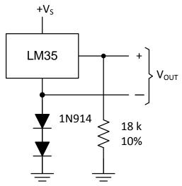
Figure 18. Temperature Sensor, Single Supply (-55° to +150°C)
