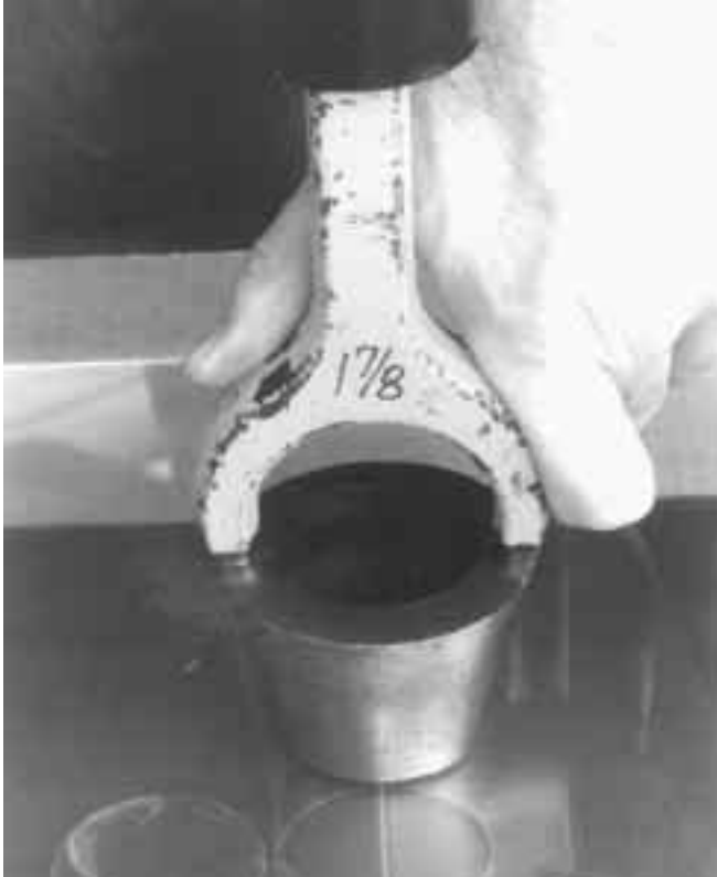
Above: Punching PEM from sheet with arch punch. Photo by Reynaldo Cortez
