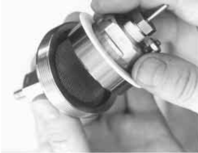
Above: Fuel cell disassembled, showing a gas distribution plate on the left. Photo by Reynaldo Cortez
