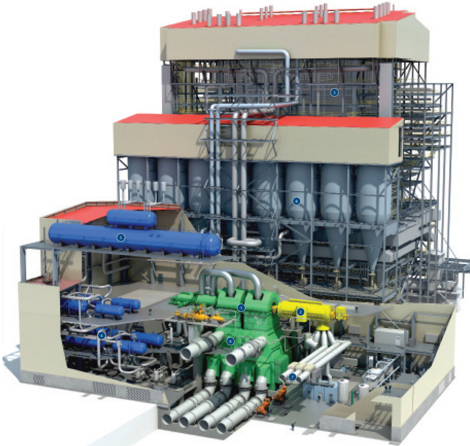
Figure 7.1: Manjung 4, A Modern 1 GW electric coal plant. Turbine(green) in the foreground. Boiler in the background.
