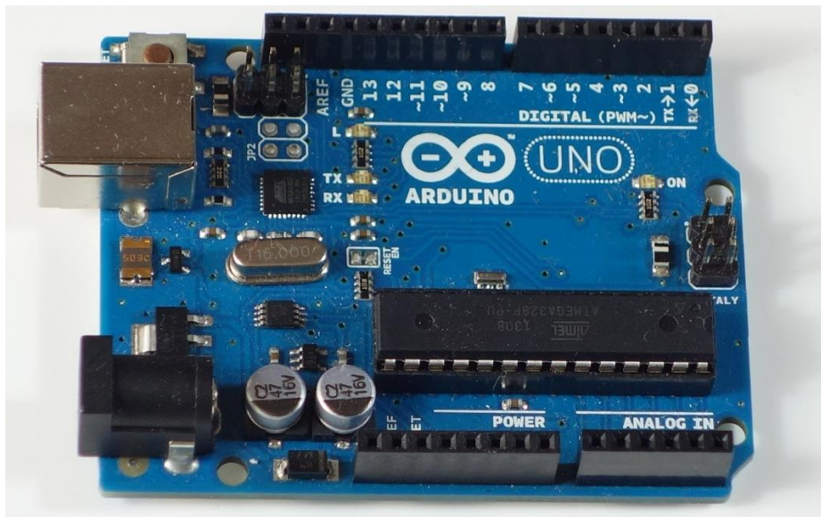
Arduino UNO R3 board with ATmega328P
