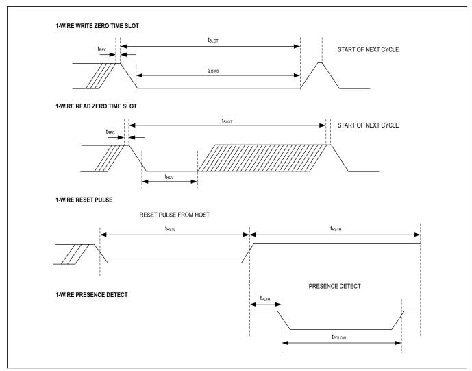
Figure 2. Timing Diagrams
