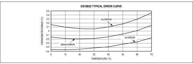
Figure 1. Typical Performance Curve
