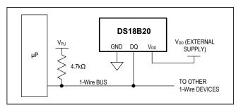
Figure 7. Powering the DS18B20 with an External Supply
