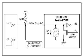
Figure 12. Hardware Configuration
