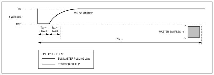
Figure 18. Recommended Master Read 1 Timing
