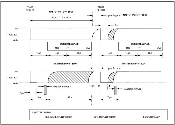
Figure 16. Read/Write Time Slot Timing Diagram
