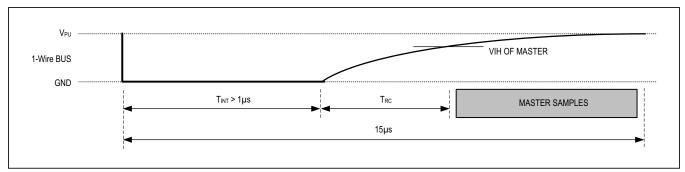
Figure 17. Detailed Master Read 1 Timing
